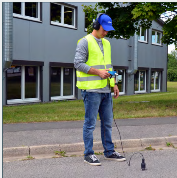
Pinpointing with HL 50-BT and PAM B-2 microphone
