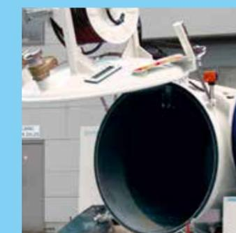
Hydraulically operated rear cover (standard model)
