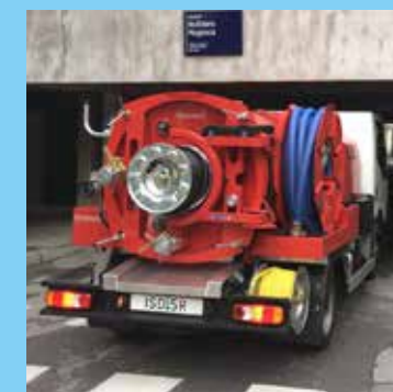
Modifications to the chassis mean that a roof height of less than 2 metres can be achieved
