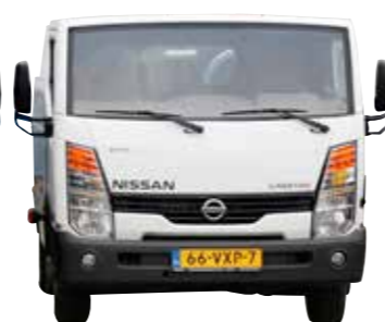
Height of 1.85 m with cab and suspension modifications
